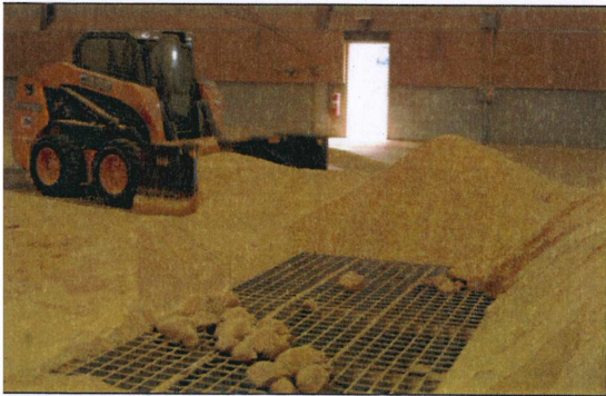
Dried distillers grains are moved to a pit for conveying to a truck for loading.
